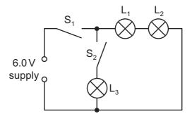
Which lamps light when switch  $S_1$  is closed and  $S_2$  is open?
