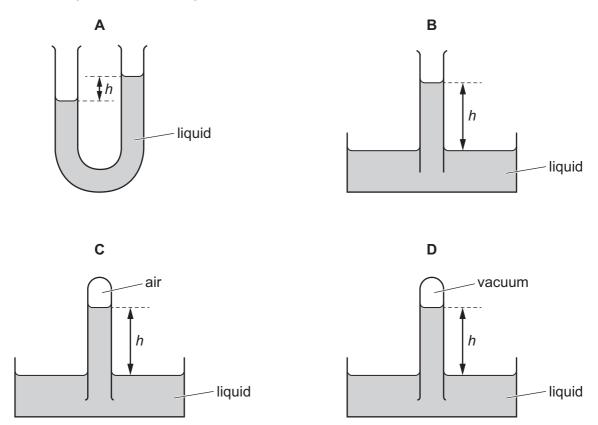
**12** A manometer contains mercury of density 14 000 kg/m³. The manometer is connected to a gas supply and the difference in the height of the mercury levels is 72 mm. The atmospheric pressure is 100 kPa.
